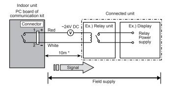
$^{\star}$  Make the distance from the PC board to the connected unit within 10m. Relay spec. : Max.24V DC, 10mA to less than 500mA
