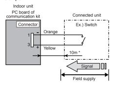
\* Make the distance from the PC board to the connected unit within 10m. Contact capacity: 24VDC or more, 10mA or more.
