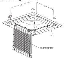
3.6. Close the intake grille, and hook the loop of the hook wire to the attached screw at step 3.3. (left and right 2 positions).
