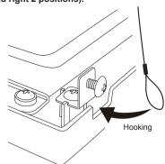
3.7. Fasten the hook wire and tighten the screw till the end. (left and right 2 positions).
