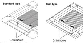
(2) Open the intake grille and remove
