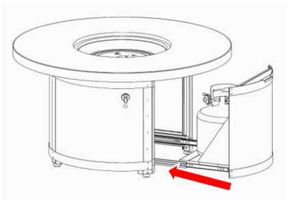
**NOTE:** Over time the bearings in the door glides may require Re-greasing. Perform re-greasing once a year to maintain the smooth operation of the slides. To re-grease the slides, spray any spray lubricant, such as WD-40, into the bearings as you slide the drawer back and forth.
