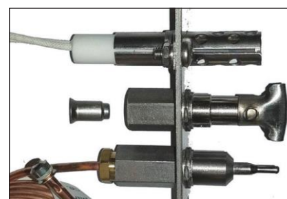
Figure 9.3 – Cleaning pilot orifice
