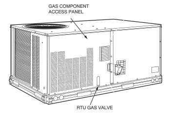
Fig. 5 – Gas Component Access Panel and RTU Gas Valve Location
