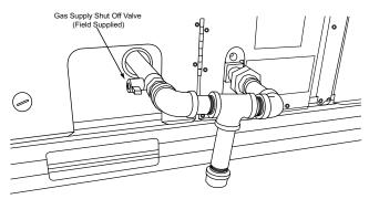
Fig. 2 – Gas Supply Shut-Off Valve (Thru the base gas supply shown.)
