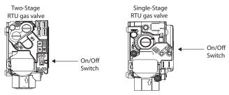
Fig. 16 - Single- and Two-Stage Gas Valves
