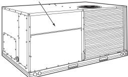
Fig. 19 – Air Filter Access Panel
