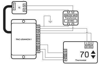
Example 3: Single-stage Cooling and Heating with Dedicated Fan Speed Relays
