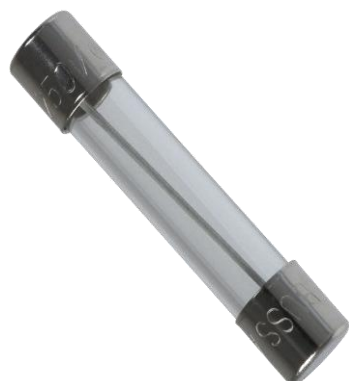
A 1-1/4 " X 1/4", 5 AMP, 120 VOLT, FAST-BLOW CARTRIDGE FUSE*
