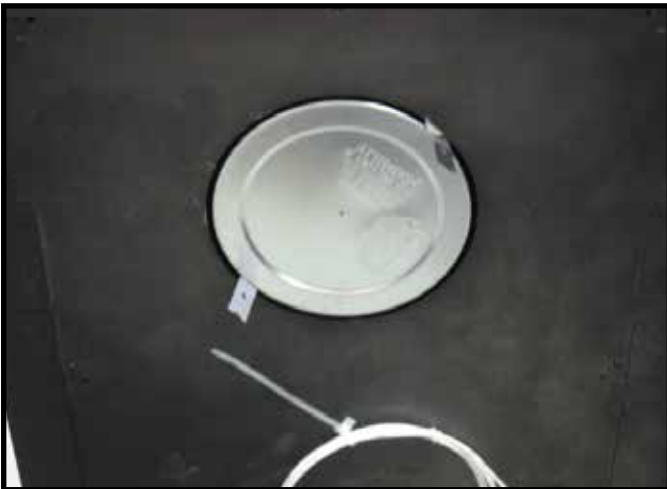
Figure 6.7 Remove the seal cap.
