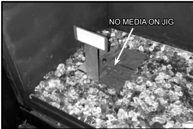
Figure 2. Media Placement Jig in Place
