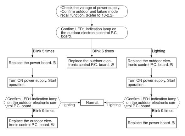
X Turn OFF power supply before removing P.C. board.
