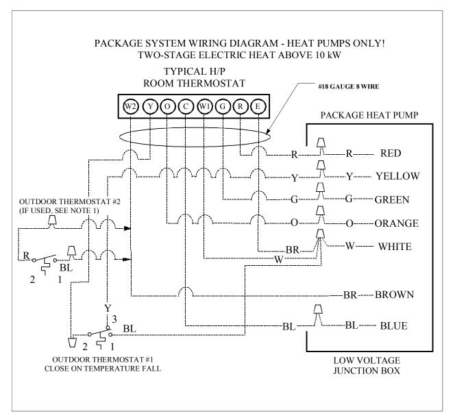
For outdoor temperatures below 0° F with 50% or higher relative humidity, set outdoor thermostat at 0° F
