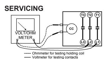
TESTING COMPRESSOR CONTACTOR (Three-phase)
