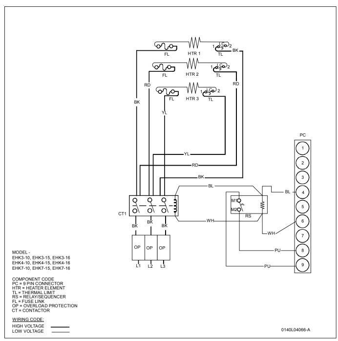
EHK3-10 HEAT KITS - 10 KW, EHK3-15 HEAT KITS - 15 KW EHK4-10 HEAT KITS - 10 KW, EHK4-15 HEAT KITS - 15 KW EHK7-10 HEAT KITS - 10 KW, EHK7-15 HEAT KITS - 15 KW
