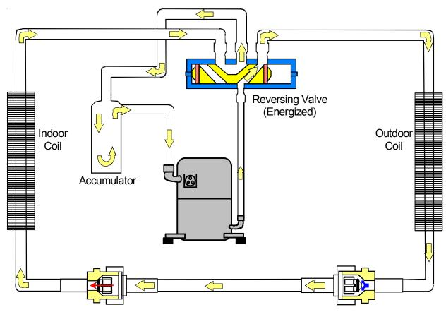
Typical Heat Pump System in Heating
