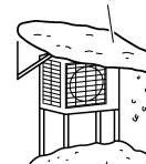
Install the unit high enough off the ground to prevent burying in snow.
