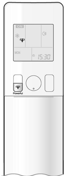
POWERFUL operation quickly maximizes the cooling (heating) effect in any operation mode. In this mode, the air conditioner operates at maximum capacity.
