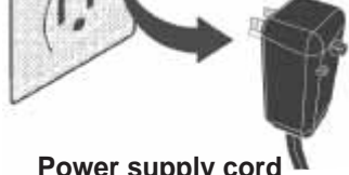
Power supply cord with 3-prong grounding plug and current detection device
