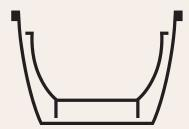
Shell and fire box each cast as a single piece of iron. Interior wall cavity reduces heat loss. Durable, weather-resistant powdercoat finish.
